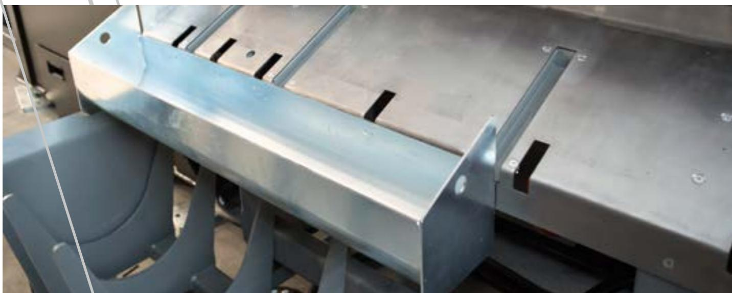
The kit for short bars enables processing bar lengths min. 50mm - 450mm. The automatic bar length setting system will also process any batch of short bar lengths in succession, avoiding down-time for length change. The kit includes a measuring ledge for short bars and a collecting box for bars shorter than 600mm. The kit for short bars is fully compatible with the automatic bar length setting system enabling short bars of different lengths to be cut in succession.
