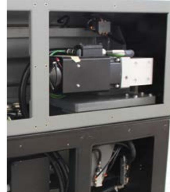
The independent servo controlled wire feed speed can reach 160m/min. and combined with the independently servo controlled rotor speed enable accurate settings to suit the diverse steel wire grades. This independent adjustment will allow flexible settings in direct relation to the diverse wire grades in order to fine-tune and obtain perfect straightness.
